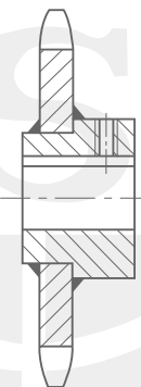
Connection by welding
